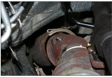
Reconnect the turbo oil drain and oil supply.
