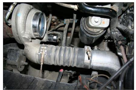
Disconnect the compressor outlet boot.
