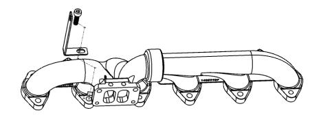
You now have the option to drill a hole through the OEM coolant pipe tab and secure the brackets together using the ¼ bolt (1100110), ¼" flat washer (1100111), ¼" lock washer (1100112), and the ¼" nut (1100113) supplied. Use a 5/16" drill bit to accomplish this.
