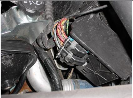
Rotate the connector so that you can remove the back plastic protective backing. Use a small pick of small screwdriver to do this.
