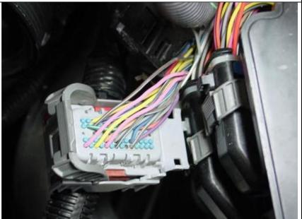
View the connector from the ECM side and ensure the pin is fully seated by comparing to adjacent pins. Lightly tug on the wire to ensure it is fully seated and locked.
