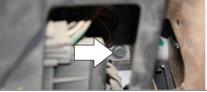
Locate suitable pass through location on firewall. Suggested location is alongside the smaller wiring harness passing through the firewall, this is located towards the passenger side of the brake booster assembly. Cut a small slit in the rubber boot using a utility knife for the wire to pass through. Alternatively, if other wires are already fed through the main wiring harness connector below the brake booster, this route may be used instead.
