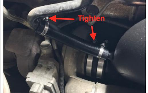
**10b.** The stop bead on the Intake Tube (B) should be sealed up to the tube seal. Slide the air filter onto the intake tube and tighten the #88 Hose Clamp (S). Align the box prongs on the bottom of the air box with the grommets on the side of battery tray and push down on the box to completely seat the prongs onto the grommet. Tighten the hose clamp at the turbo and CCV line.
