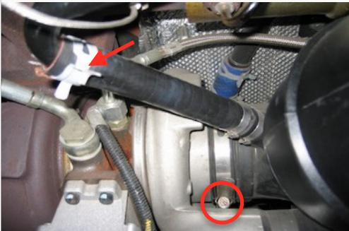
4. Remove the mounting nut on the stock air box. Save the nut for the installation.
