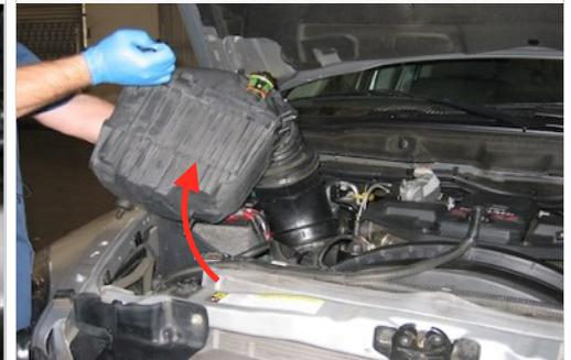
6. Install the Tube Seal (C) onto the Air Box (A).
