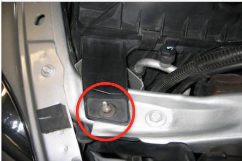
5. Lift up and out to remove the stock air box assembly from the vehicle.
