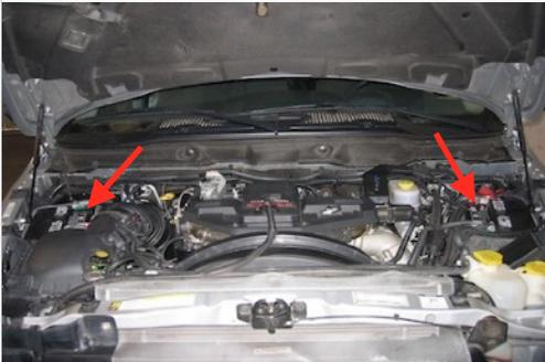
2. Disconnect the electrical harness connectors for the Intake Air Temp (IAT) and the Mass Air Flow (MAF) sensor then unsnap the wire loom from the tube. On the MAF sensor, slide the **red** locking tab up then press down on the tab and pull the connector out. For the IAT sensor, press down on the grey tab and pull the connector out.
