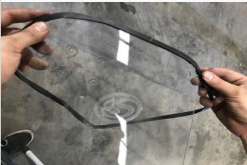
**14.** Place the Clear Lid (I) on top of the Air Box (A) using the supplied 10-24 Screws (L) and Washers (K).
