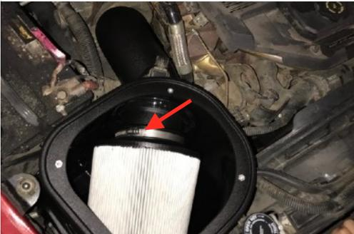
**11.** Secure the Air Box (A) using the stock mounting nut removed in Step #4.
