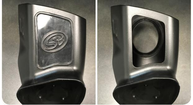
**9** Carefully remove the MAF sensor from the stock intake tube then install the sensor onto the Intake Tube (C) with the 8-32 Screws (M), MAF Plate (H) and MAF Gasket (G). Install the Filter Minder Grommet (J) into the intake tube.
