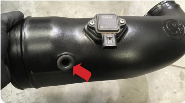
**10** Slide the Coupler (F) and #56 and #52 Hose Clamps (P & N) onto the Intake Tube (C). Make sure the coupler is seated up to the stop bead. Tighten the #56 hose clamp only, leave the #52 hose clamp loose.
