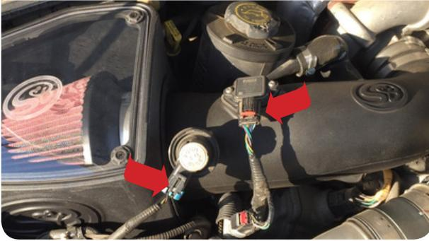
**19** Reconnect the negative terminal on both batteries. Inspect your installation, make sure the kit is properly positioned and all fasteners are secure. Keep all stock parts in case you would ever need to reinstall the stock intake assembly. Affix the ID label near the intake kit. The installation is now complete.
