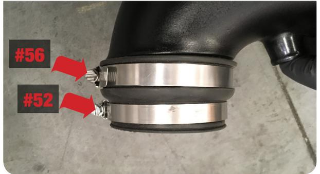
**11** Install the Intake Tube (C) into the Air Box (A) then install the intake assembly into the truck. Align the fender side opening of the airbox with the inlet, then rock the airbox downward. Push down on the box to make sure that the air box is completely seated on the grommets then slide the coupler onto the turbo inlet.
