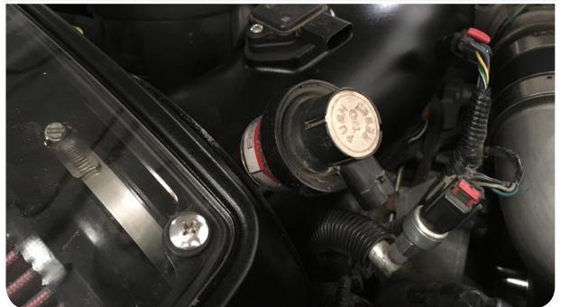
**18** Reconnect the MAF sensor harness into the MAF sensor and engage the red locking clip. Reconnect the sensor harness into the filter minder.
